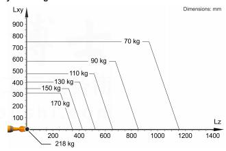
The KR 150 R2700-2 F is designed for a rated payload of 150 kg in order to optimize the dynamic performance of the robot. With reduced load center distances, higher loads up to the maximum payload may be used. The specific load case must be verified using KUKA.Load. For further consultation, please contact KUKA Support.
